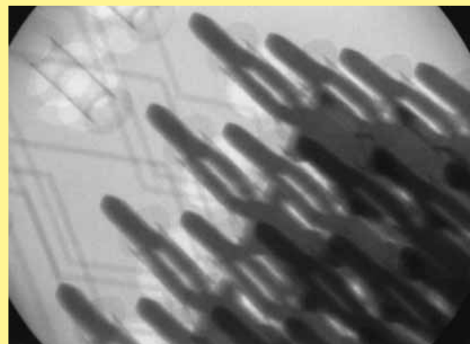
X-ray photo of a pressed-in connector
